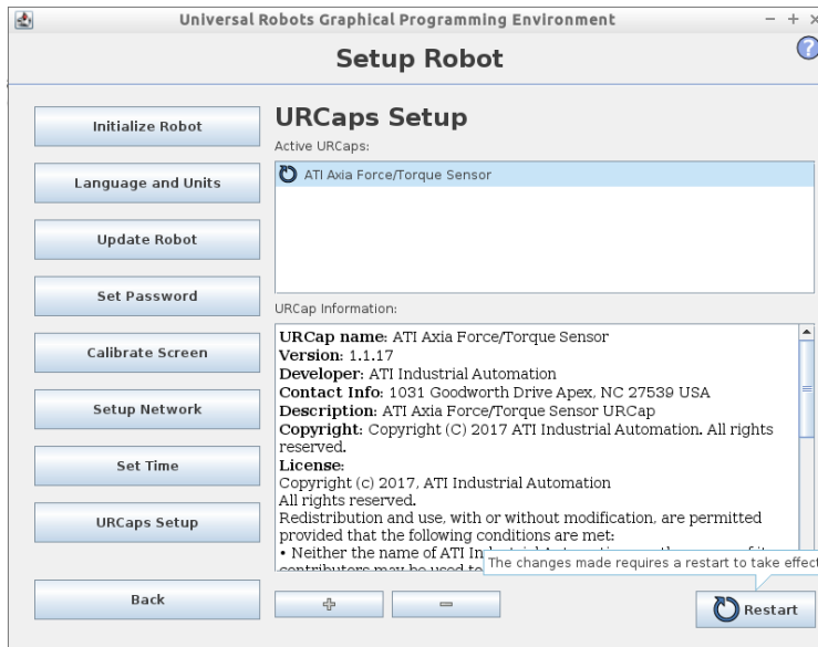
Figure 3.6—Finish Installation of the URCaps Software
